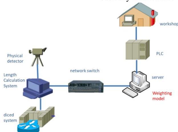
**Figure1.** Schematic diagram of fixed weight model and weighing system
