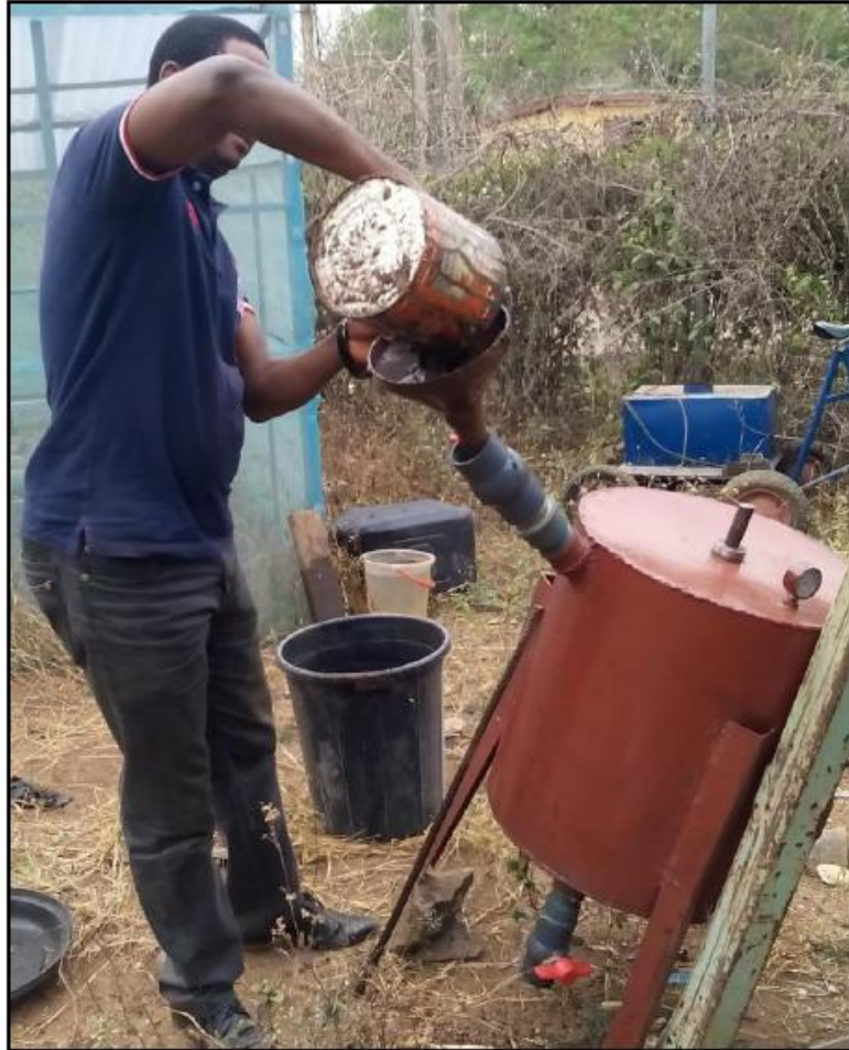
Plate2. Loading of Biogas Digester with Mixed Substrates
