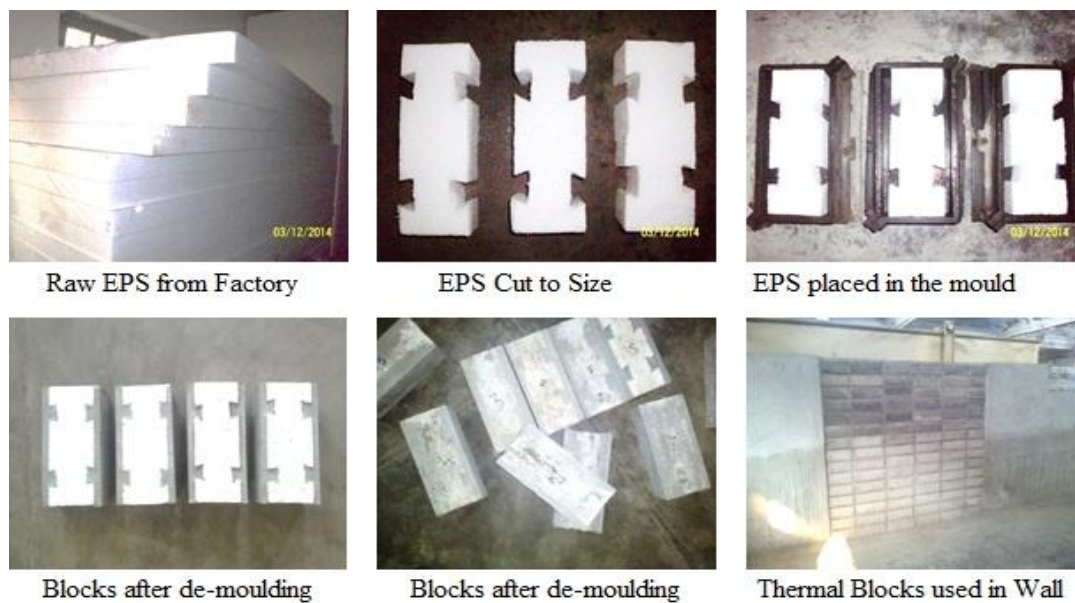
Figure2. Making process of thermal blocks
