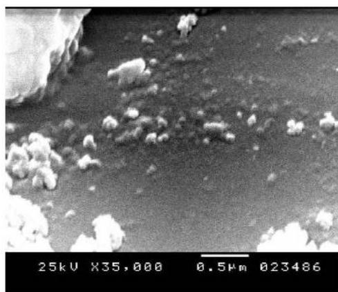
**Figure7.** SEM image of Nano-SnO<sub>2</sub> at magnification order = 35,000x
