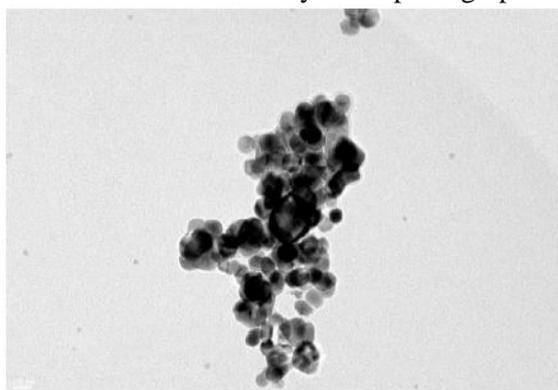
Figure3. HR-TEM image # 1 of Nano-SnO<sub>2</sub> at magnification order
