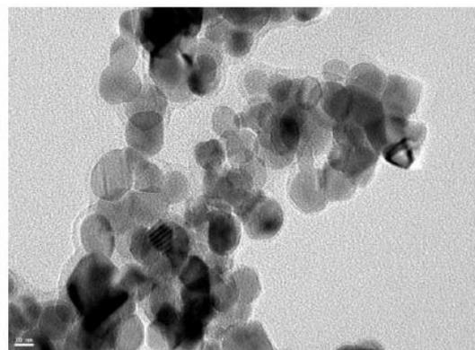
Figure6. HR-TEM image # 3 of Nano-SnO<sub>2</sub> at magnification order
