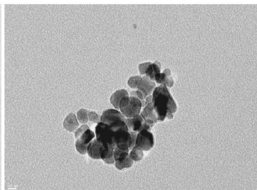
Figure4. HR-TEM image # 2 of Nano-SnO<sub>2</sub> at magnification order
