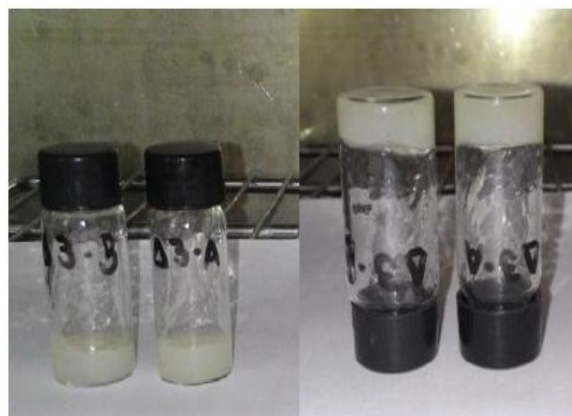
Figure 9. Images of oxidized citrus pectin hydrogel gelification in the presence of adipic acid dihydrazide, at pH 3.0.
