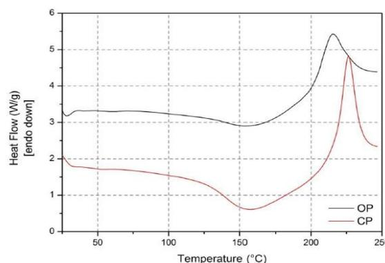
**Figure8.** DSC thermograms of citrus pectin (red curve / CP) and oxidized citrus pectin (black curve / OP).
