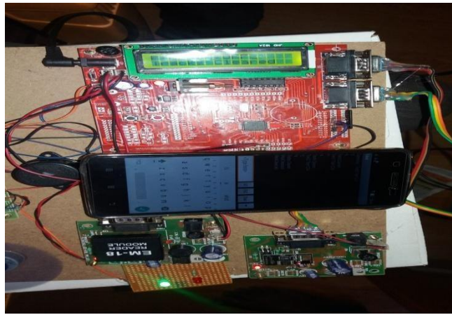
Fig4. Track Cleared Message Displayed on LCD When Train Went Out on Track
