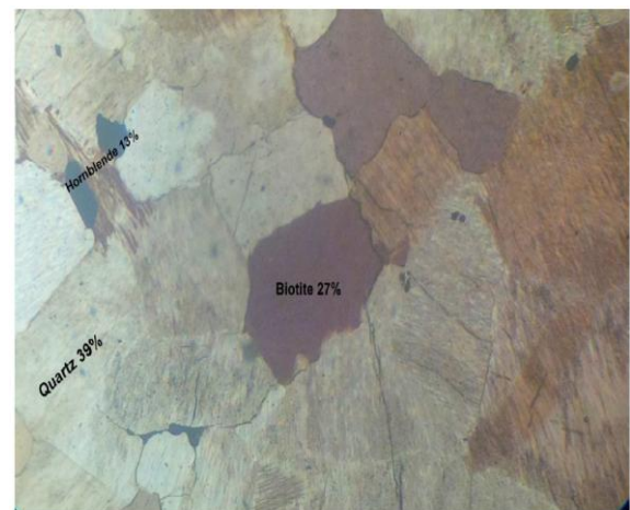
Plate 3: petrography of ado/ikere road charnockite rock (sample 3)
