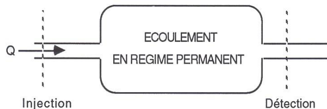
Fig2. General principle of radiotracer application in industry.
