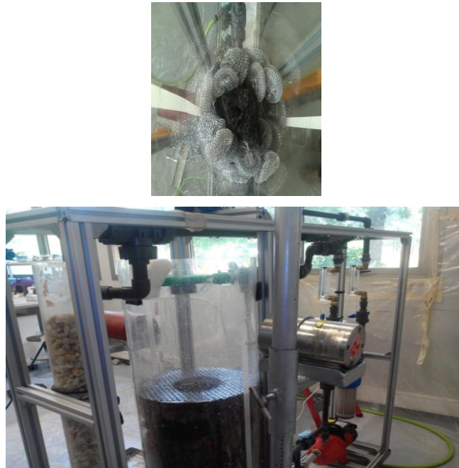
Fig3. Constructed laboratory on packed bed accompanied by the sealed source and detector
