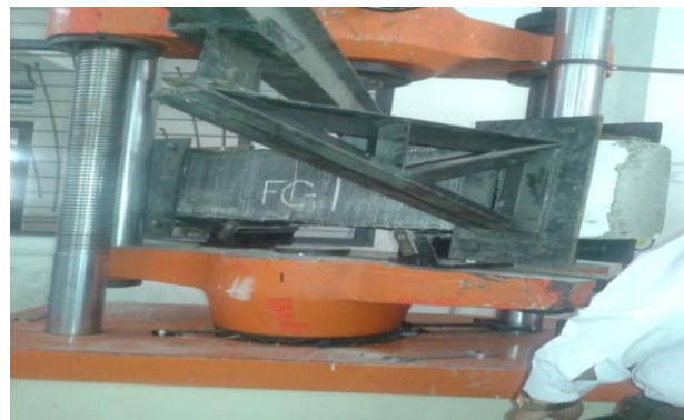
Fig4. The beam wrapped with carbon fibre for testing
