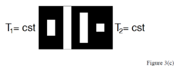
Figure 3. Cavity and substrate sections: a) Series arrangement. b) Parallel arrangement. c) Hybrid arrangement (combination of the series and parallel arrangements). Hybrid arrangement was shown for demonstration and consisted of four cavity and five substrate sections. Dark shades are the substrate sections and white regions are the cavities or materials of different \kappa values.
