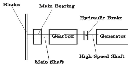
Figure 5.2. Turbine components layout
