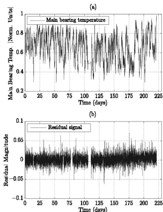
**Figure 5.7.** Main bearing temperature and residual signal (Turbine A)
