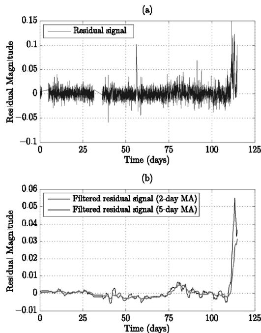
**Figure 5.10.** Main bearing temperature residual and filtered residual signal (Turbine B)
