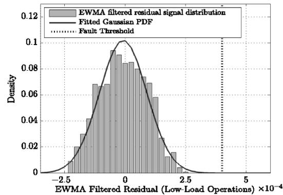
**Figure 5.13.** Distribution of EWMA filtered residual signal during Low-Load operations for 3 fault-free turbines
