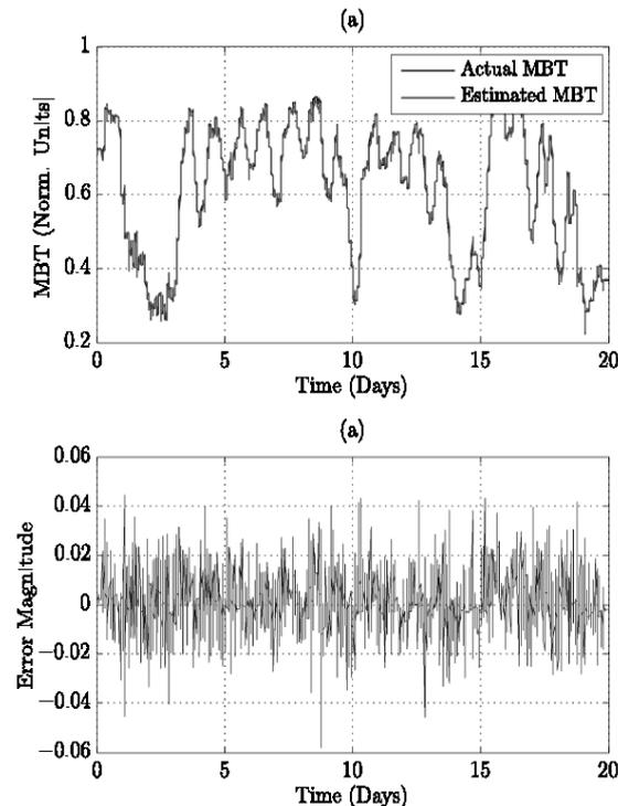
**Figure 5.5.** Main bearing temperature estimation (a) and generated residual signal (b) indicating error magnitude at each sample time (fault-free turbine)
