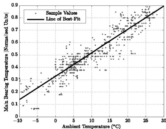
**Figure 5.3.** Relationship between main bearing temperature and ambient temperature, under low-load conditions
