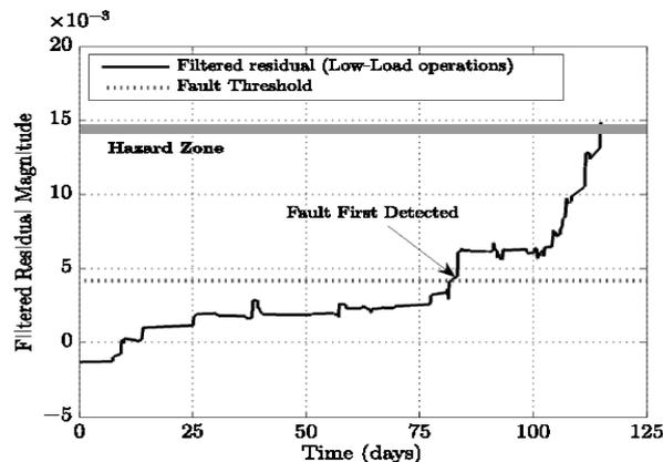
**Figure 5.14.** Evolution of EWMA filtered residual signal during Low-Load operations for faulty main bearing (Turbine B)
