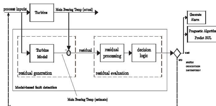
Figure 5.1. Main bearing model-based condition monitoring algorithm
