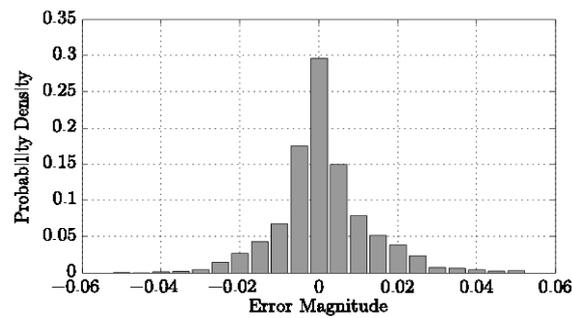
**Figure 5.6.** Distribution of residual signal between estimated and actual main bearing temperature (fault-free turbine)
