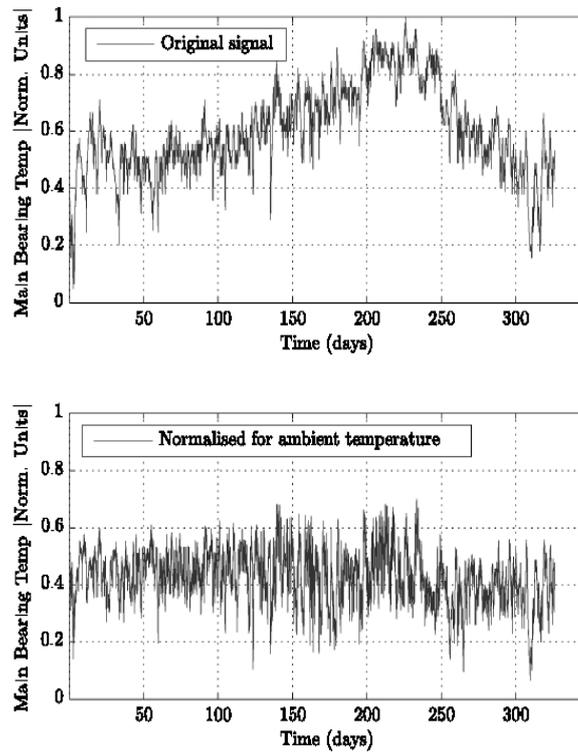
**Figure 5.4.** Main bearing temperature: original signal ((a) upper plot) and normalized for ambient temperature signal ((b) lower plot)
